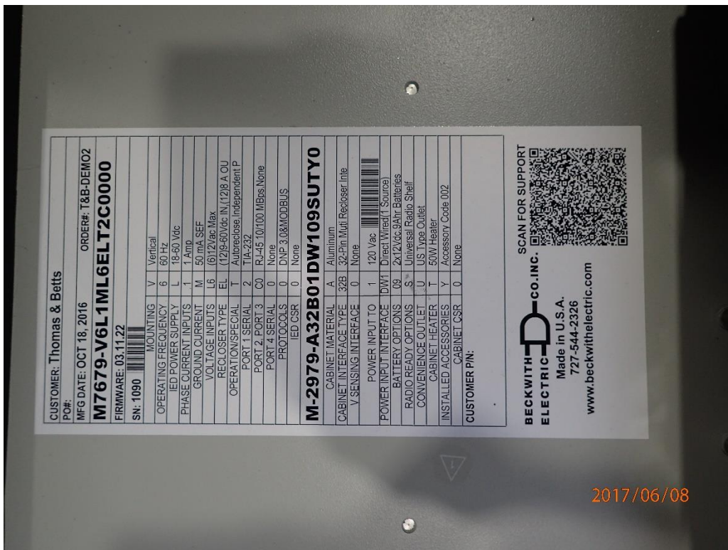
Figure 18: Nameplate of the tested recloser controller.
