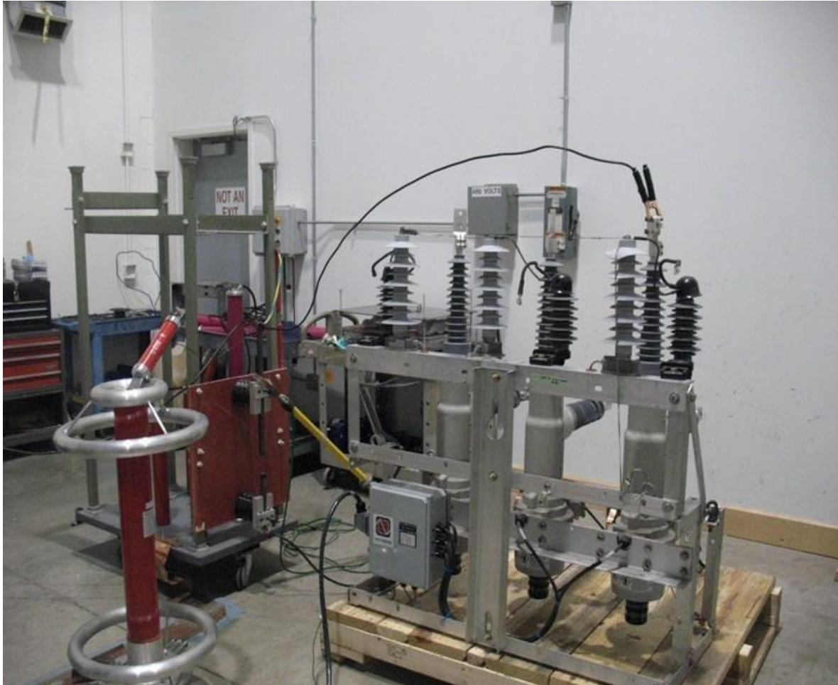
SSAO Recloser test setup
