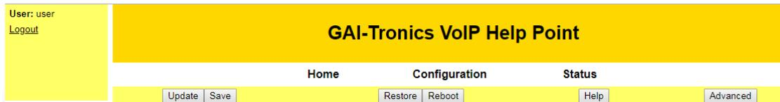
All the web pages in the telephone have a common header section showing the name of the device, the current user name, links to the 3 main sections (Home, Configuration & Status), and controls for the configuration process (Update, Save, Restore, Reboot etc).
