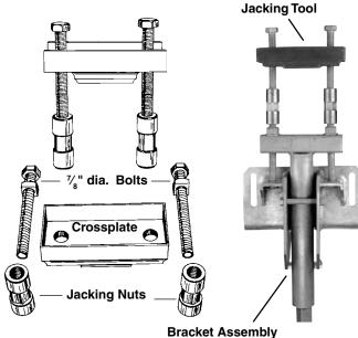
12. Place the jack or hydraulic cylinder between the T-Pipe and the cross-plate on the jacking tool. Adjust the height of the jacking tool as required to meet the height of the jack.
