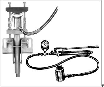
13. Apply a small amount of pressure to the jack, just enough to take up the "slack" in the assembly. Once again, check to see if the bracket is still mounted flush with the foundation. Tighten the cross-bolt if necessary and check the bracket mounting bolts again before proceeding.
