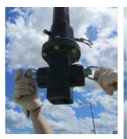
4. With the release rings in the outside position, insert the Drive End Assembly into the Locking Dog Assembly. Rotate rings to the inside position to capture drive end in the Locking Dog Assembly.
