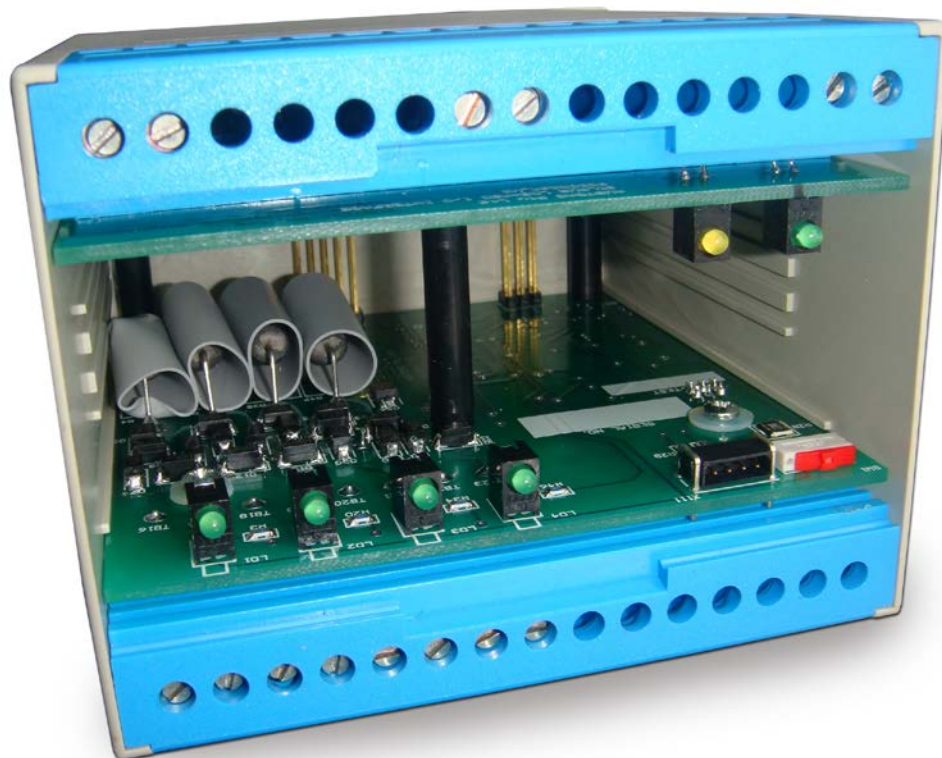
Photograph 2 Access to console port and programming switch
