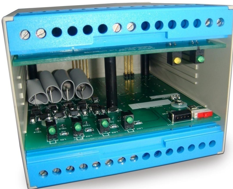
Photograph 2 Access to console port and programming switch
