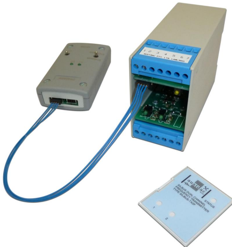
Photograph 4 SILBUS-TX2F console port connected to MEAN1 interface
