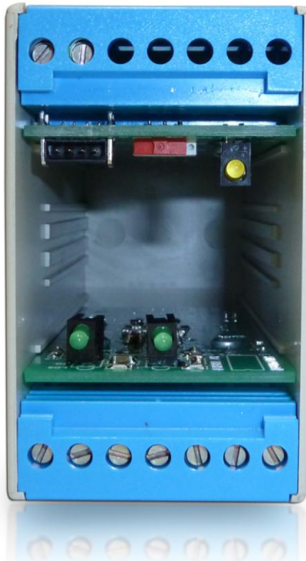
Photograph 2 Access to console port and programming switch
