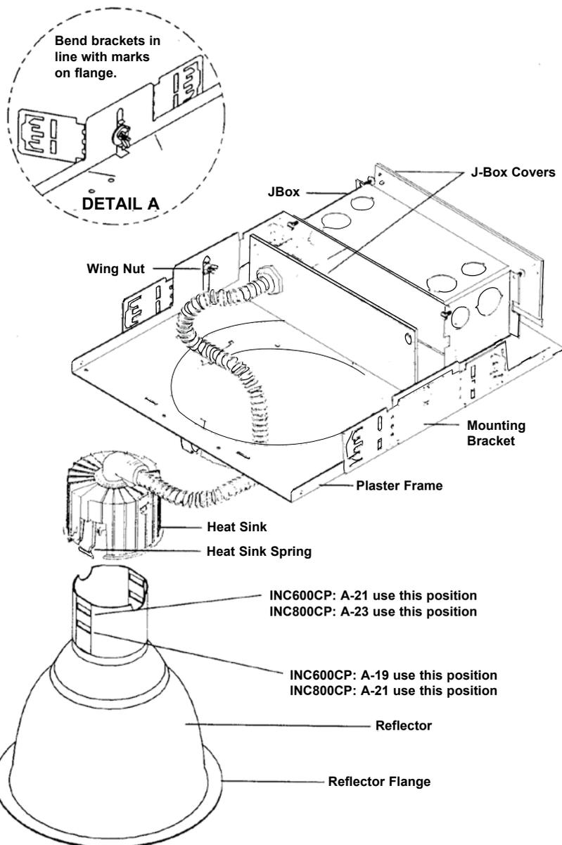
**CAUTION: DO NOT ATTEMPT TO MODIFY OR REWIRE FACTORY-INSTALLED WIRING ON THE FIXTURE. SAFETY AND PROPER OPERATION OF THE FIXTURE DEPEND ON THE INTEGRITY OF THE WIRING.**
