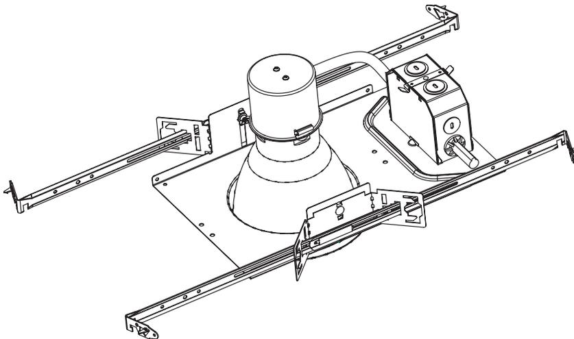
1. Disconnect hanger bars and brackets and re-install as shown. Install the fixture in the ceiling using hanger bars (supplied), or mounting channel or bar (by others) placed in the adjustable mounting brackets. Mount the fixture in the ceiling so that the weight of the fixture is supported by the hanger bars, mounting channel, or bar and/or hanger wires secured to the building structure.
