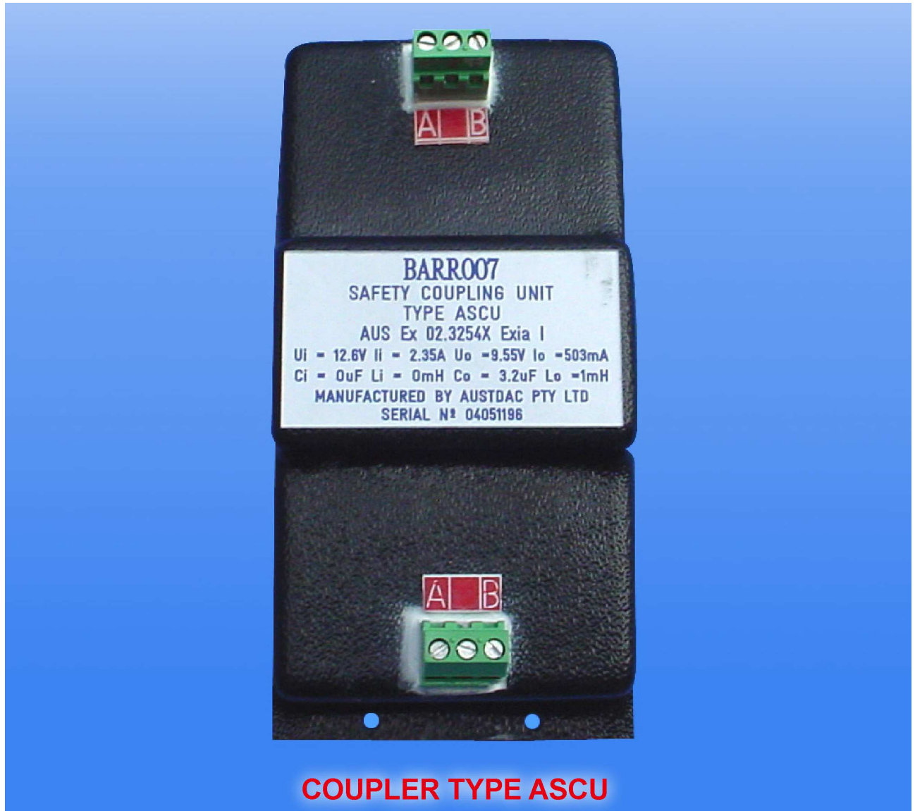
Photograph 19. Coupler type ASCU front view.
