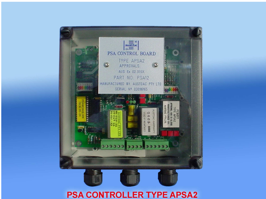
Photograph 2 Pre-start alarm controller type APSA2 front view
