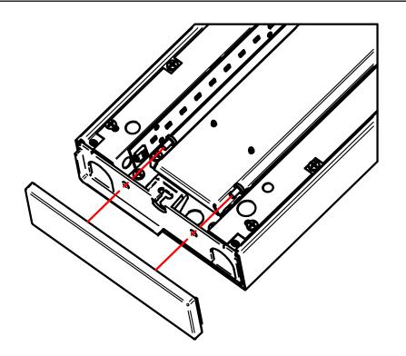
Install end caps by sliding into end headers and attaching with two 10-32 machine screws (provided).
