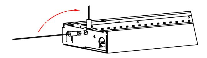
Pre-hang FAI kits and feed drops then insert single point suspension nuts into end hanger to mount fixtures on to ceiling. Refer to Suspension instruction sheet 510481.
