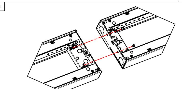
For row mounted fixtures, slide the end headers into their respective slots and attach with two 10-32 machine screws and hex nuts (provided).
