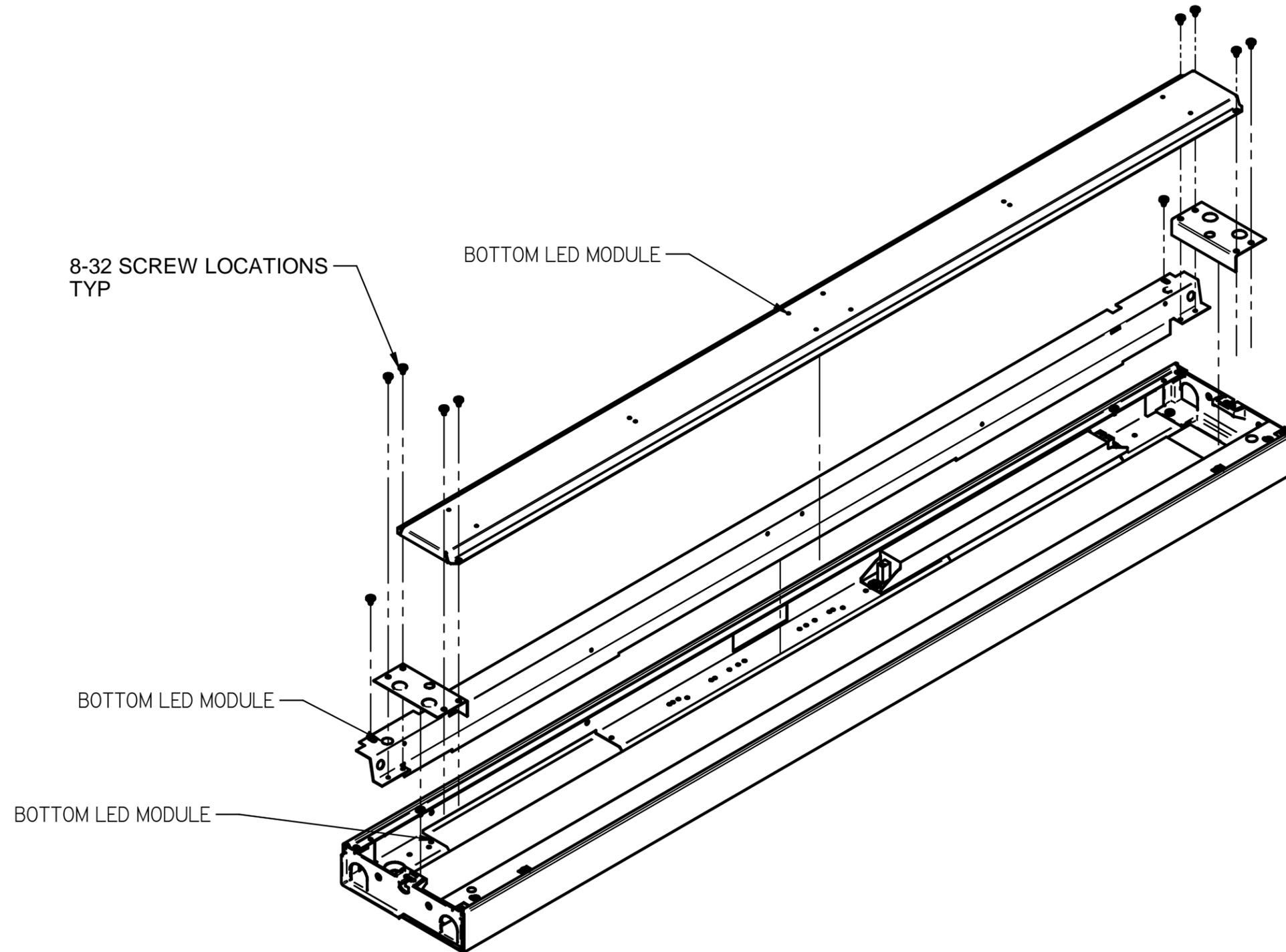
1. Remove four 8-32 screws to remove bottom LED module
