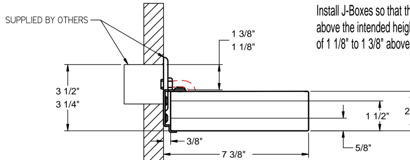
Install J-Boxes so that the top of the openings are 3 1/4" to 3 1/2" above the intended height of the fixture. This will give a J-Box opening of 1 1/8" to 1 3/8" above the top of the wall bracket/fixture.
