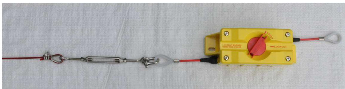
Photograph 6 ESS3 Pullkey with Tension Setup
