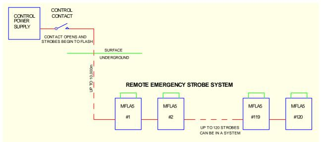
Figure 3. Remote emergency strobe system
