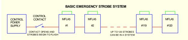
Figure 2. Basic emergency strobe system
