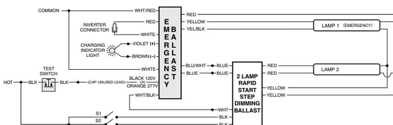
THE WHITE/BLACK LEAD MUST CONNECT TO THE WHITE LEAD OF THE STEP-DIMMING BALLAST ASSOCIATED WITH THE EMERGENCY BALLAST ONLY. CONNECTIONS TO OTHER BALLASTS OR FIXTURES COULD RESULT IN ABNORMAL OPERATION AND CAUSE PRODUCT DAMAGE.
