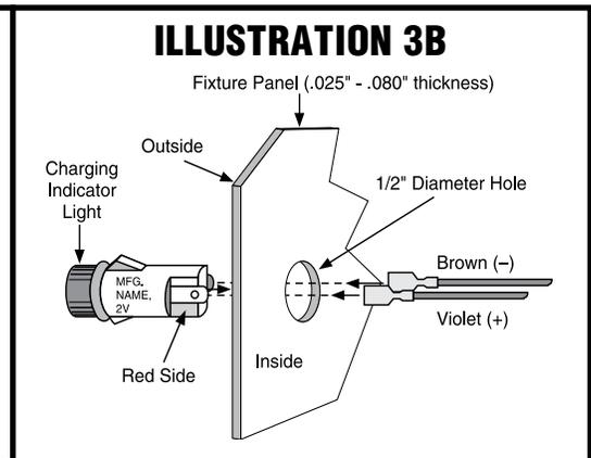
NOTE: After installing the charging indicator light and test switch, mark each with the appropriate label. If a detached charging indicator light is used, connect by matching wire colors and install as shown on the installation insert page.
