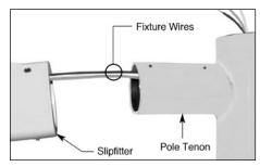
**1.** Pull field wires through the pole tenon and slipfitter into the housing. Carefully slide the slipfitter over the tenon, making sure wires are not pinched.
