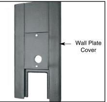
3. Caution: Structural integrity of mounting plate attachment to wall is by others. The fixture arm cover plate assembly is hooked to the wall mounting plate and secured with stainless steel screws provided. Field splices are made at the opening in the cover plate. (See Fixture Wall Mount Installation Instructions)
