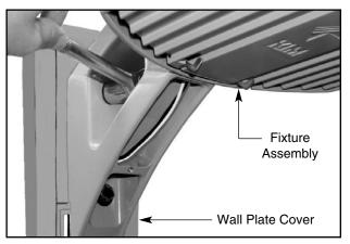
3. Attach fixture assembly to wall plate cover (2 places) using washer and 3/8" bolt. Tighten to 20 ft.-lbs. using %16" socket wrench.
