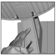
6. Tuck wires in and install arm access cover. Secure with flat head screw using a 1/8" allen wrench.
