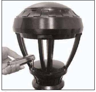
To install base casting to pre-set anchor bolts, base casting must be removed from fixture. Remove the 2 screws from splice compartment cover using ½" hex wrench.
