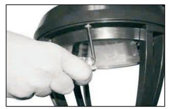
3. Close hood assembly and tighten screw.
