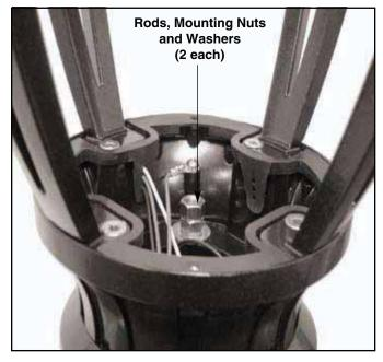
2. Remove the nuts & washer from the mounting rods using a %6" deep socket, ratchet & extension.
