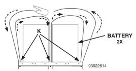
Place front batteries in between middle and front "K" anchors and thread straps OVER batteries as shown in **Fig. 7.**
