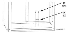
Install all (6) strap anchors "K" with screws "B" supplied in kit shown in Fig 5.
