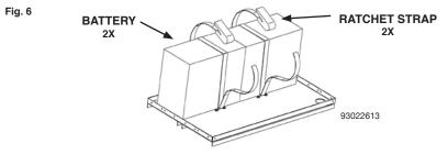
Thread straps through back and middle anchors and place OVER batteries as shown in Fig 6. NOTE: No part of straps should be under batteries.
