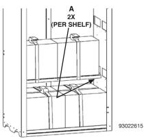
Once the batteries are strapped down on the bottom of the cabinet, place the first shelf in the lower back position and secure it with sheet metal screws "A" provided, one per each end of the shelf.
