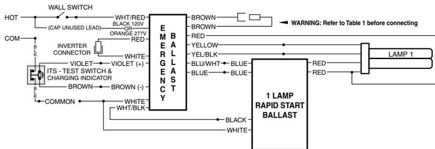
**WIRING DIAGRAM for Emergency-Only fixtures**
