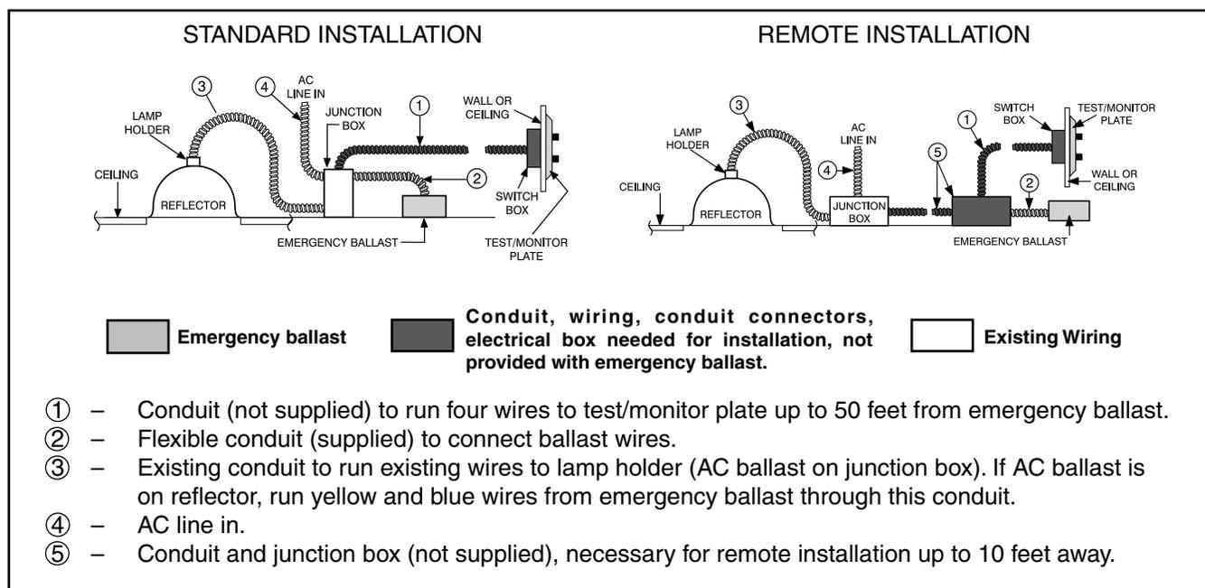
4. See back page for more detailed wiring schematics. The emergency ballast can be used with one- or two-lamp fixtures, and operates one lamp in the emergency mode.
