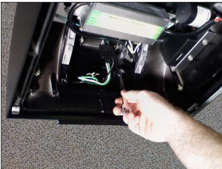
7. Tighten nuts inside housing 5-8 ft. lbs.
