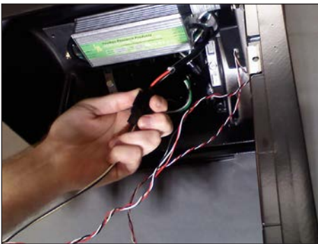
10. Join the disconnect plugs between the emitter deck assy and driver assy.
