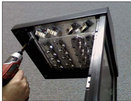
11. Install emitter deck into housing making sure all screws protrude through keyhole slots and tighten screws. Close lens frame to complete installation.
