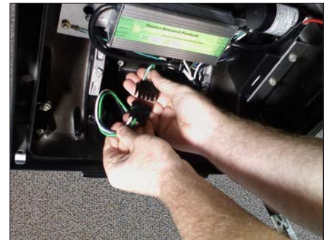
9. Join the disconnect plugs between the power lead-in and the driver assy.
