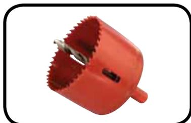
Use a 2 7/8" hole saw and pilot drill to cut an opening for the D2LED downlight. Because of the small reflector flange of the D2LED, the accuracy of this hole is critical. Even a 3" hole saw may leave a ceiling cut out too large to be completely hidden after installation.
