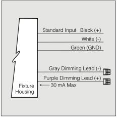
Driver has a 0-10V dimming interface with a dimming range of 10-100%. Is compatible with most control systems including Hubbell Building Automation wiHUBB<sup>™</sup>. Approved dimmers include Lutron Diva AVTV, Lutron Nova NFTV and NTFTV. Note: Not compatible with current sourcing dimmers. Controls compatible via Gray and Purple dimming lead.
