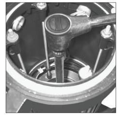
**5.** Tighten securely using 9/16" socket with a 12" extension and ratchet
