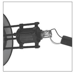
**3.** Feed fixture wires down pole and out hand hole in pole.
