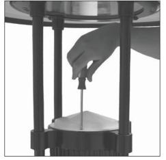
6. Secure the driver housing cover to fixture using a Phillips screwdriver.
