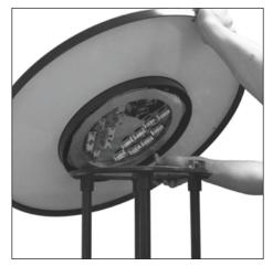
**3.** Hold the hood up with your left hand, push the stop arm straight back to release.
