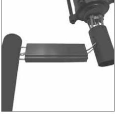
**2.** Feed supplied wiring through round fitter, arm, wiring hole in pole and out hand hole.
