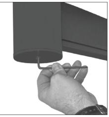
1. Install pole and arm cap using a 7/64" allen wrench.
