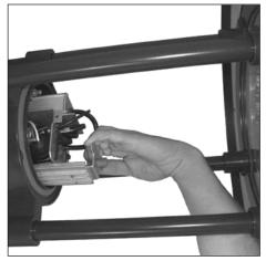
**2.** Grab handle and slowly remove driver assembly. Make sure wiring does not catch.
