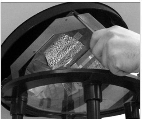
**7.** Remove (2) front screws securing reflector assembly to fixture hood and lift free of lower locating pins.
