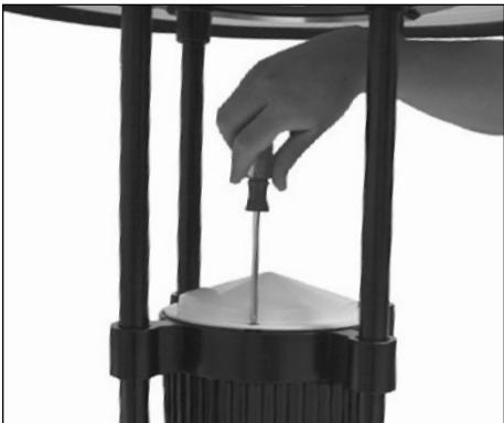
**1.** Remove electronic driver cover from fixture.
