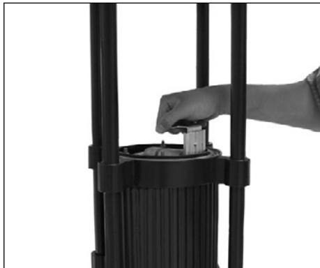
**2.** Grab handle and remove HID ballast assembly from the housing.
