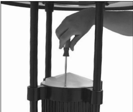
**4.** Install driver housing cover and tighten securely.
