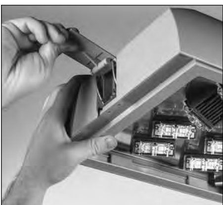
15. Push up on door frame and push latch lever up and inward. Swing latch down to secure the door frame.
