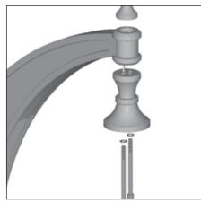
Pull wires through arm and adapter. Install adapter base & finial cap to arm with washers and screws using a 5/16" Allen wrench. Tighten to 20 ft. lbs.
