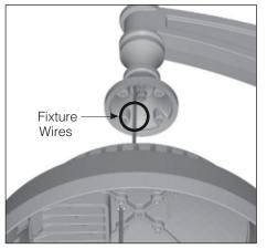
Attach fixture to arm with washers and bolts. Keep wires tight to avoid pinching. Tighten progressively until tight.
