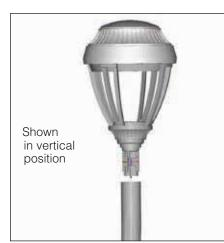
1. Lay pole horizontal on padded supports to protect finish. Pull field wires through pole and spreader into fixture splice compartment. Install fixture onto pole and tighten spreader to 20 ft.-lbs. torque.
