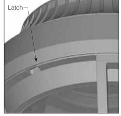
**5.** Depress latch to open and gently swing down lens frame assembly for EmitterDeck and electronic driver access.
