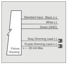
Driver has a 0-10V dimming interface with a dimming range of 10-100%. Is compatible with most control systems including Hubbell Building Automation wiHUBB<sup>™</sup>. Approved dimmers include Lutron Diva AVTV, Lutron Nova NFTV and NTFTV. Note: Not compatible with current sourcing dimmers. Controls compatible via Gray and Purple dimming lead.
