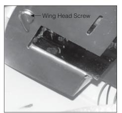
**4.** Swing electronic driver assembly into fixture and secure with wing-head screw.
