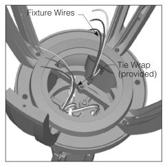
2. Thread field wires through tie wrap (provided) and back loop the wires. Connect fixture wires to field wires observing polarity; i.e., green-toground, white-to-common, and blackto-voltage.
