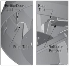
**2.** Remove the EmitterDeck by unhooking the tab on the front and slide it out of the rear bracket.
