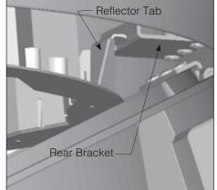
**5.** Install EmitterDeck by inserting into rear bracket and lay EmitterDeck assembly in lens frame.
