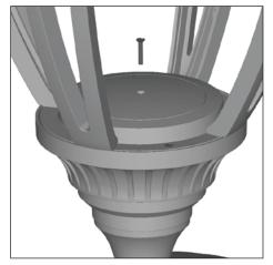
**3.** Install splice cover using screw provided.
