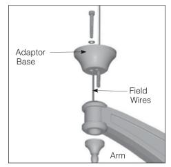
1. Pull wires through arm and adapter. Install finial or cap. Install adapter base to arm with bolts and washer supplied. Torque to 20 ft. lbs.
