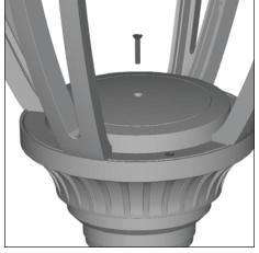
**4.** Install splice cover onto fixture using screw provided.
