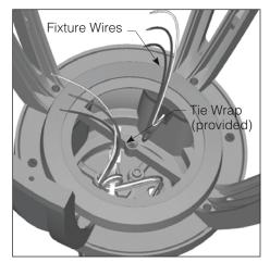
**3.** Loop wire through tie-wrap to prevent wires from disconnecting. Connect fixture wires to field wires observing polarity; i.e., green-to-ground, white-to-common, and black-to-voltage.
