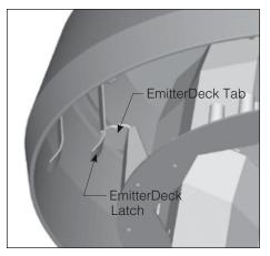
Swing EmitterDeck into housing & secure EmitterDeck tab into the front EmitterDeck latch.
