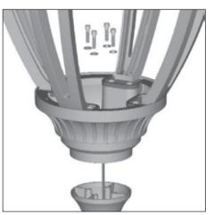
**2.** Insert field wire into fixture splice compartment. Install fixture onto adapter base with the four washers and screws using a 3/16" Allen wrench. Tighten progressively until tight.
