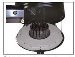
2. Unlatch ¼-turn faster on bezel assembly. Swing the bezel assembly open. Disconnect all wiring connecting bezel assembly to driver assembly and remove bezel assembly from hinge hanger.
