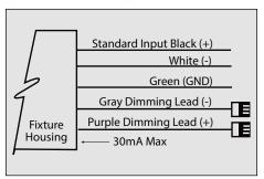
Driver has a 0-10V dimming interface with a dimming range of 10-100%. Is compatible with most control systems including Hubbell Building Automation wiHUBB™. Approved dimmers include Lutron Diva AVTV, Lutron Nova NFTV and NTFTV. Note: Not compatible with current sourcing dimmers. Controls compatible via Gray and Purple dimming lead.
