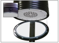
1. Open lens frame by loosening self-retaining ¼-20 screws; swing lens frame open until the stop arm prevents further movement.
