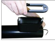
**5.** Slide support arm, arm spacer, and gasket over draw bolts. NOTE: Arm will have a circular end to fit a round pole.
