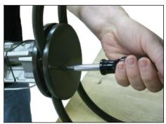
1. A wiring chamber is included at the center of the lens frame. Remove the splice cover by loosening the self-retaining screw; pull the fixture wires out into the clear area.
