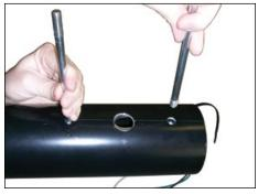
4. Insert pole-backing plate through top of pole. Align three holes in pole with matching holes in backing plate. Insert both draw bolts into pole holes and thread draw bolts into the backing plate.
