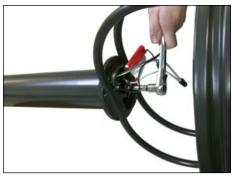
**4.** Tighten the center bolt to 25 footpounds torque. When tight, push the connected wire ends back into the chamber and replace the splice cover.
