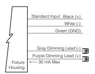
Driver has a 0-10V dimming interface with a dimming range of 10-100%. Is compatible with most control systems including Hubbell Building Automation wiHUBB™. Approved dimmers include Lutron Diva AVTV, Lutron Nova NFTV and NTFTV. Note: Not compatible with current sourcing dimmers. Controls compatible via Gray and Purple dimming lead.
