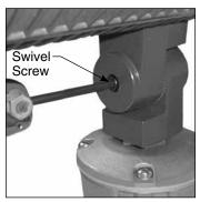
4. To adjust backtilt up to maximum, loosen swivel screw being careful not to disengage threads. Hold fixture at desired angle and firmly tighten swivel screw.
