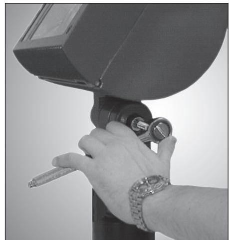
3. Loosen hex bolt to adjust fixture angle. Adjustments are in 5° intervals
