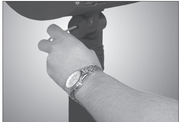
4. Adjust fixture to desired angle. Adjustments are in 5° intervals.
