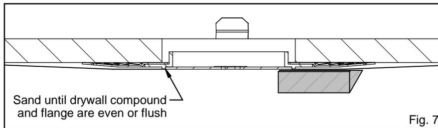
8. After drywall compound has fully cured, the ceiling can be painted. After paint has dried remove the plaster plug and any extra drywall compound or paint that may have seeped past the plaster plug by carefully scraping as required.
