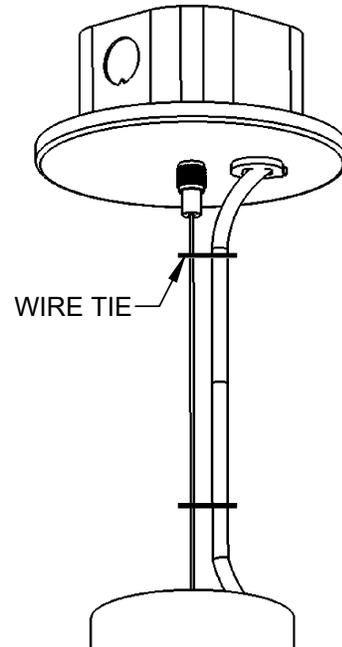
7. PLACE WIRING CONNECTIONS IN OUTLET BOX & RE-SECURE CANOPY AGAINST CEILING WITH BARREL COUPLER.
