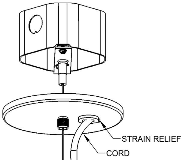
5. INSTALL CORD TO CANOPY BY UNSCREWING BARREL COUPLER & INSERTING CORD INTO BLACK OR WHITE STRAIN RELIEF & PRESSING INTO CANOPY. MINIMUM LENGTH OF 6" REQUIRED FOR CONNECTIONS.
