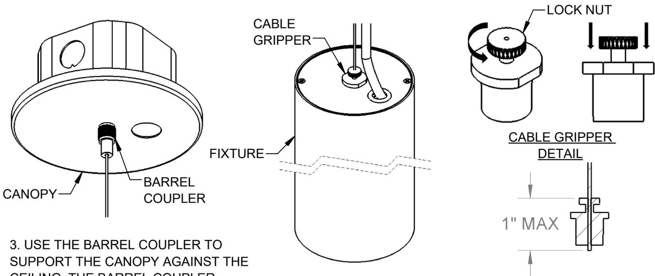
3. USE THE BARREL COUPLER TO SUPPORT THE CANOPY AGAINST THE CEILING. THE BARREL COUPLER ATTACHES TO THE CABLE COUPLER.
