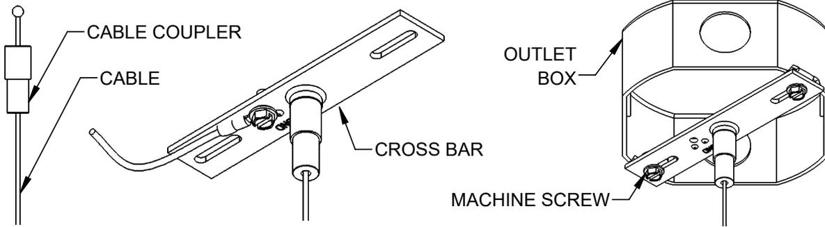
1. FEED THE CABLE THROUGH THE CABLE COUPLER & ATTACH TO CROSS BAR SCREW
