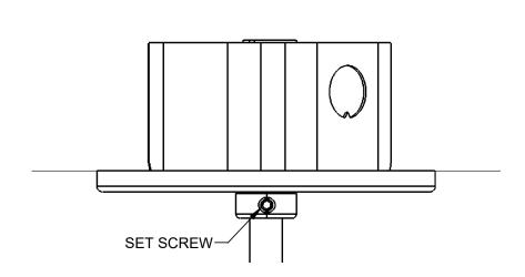
6. POSITION CANOPY AGAINST CEILING & SECURE WITH SLIP-RING SET SCREW. NOTE: FOR SQUARE CYLINDER, CANOPY SHALL BE CONCENTRIC WITH
