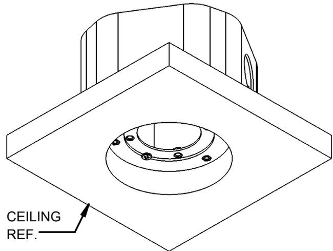
1. SECURE PENDANT BRACKET TO 4" OCTAGONAL OUTLET BOX (SUPPLIED BY OTHERS) USING (2) #8-32 FLAT HEAD MACHINE SCREWS.
