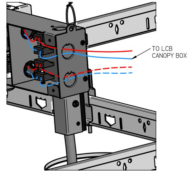
FEED ONE END OF A 18 GA SOLID **PLENUM RATED WIRE, SUPPLIED BY OTHER** INTO ENCLOSURE AND WIRE AS LABELED. FEED OPPOSITE END THROUGH LCB KO. DEPENDING ON YOUR FIXTURES NEEDS, THERE MAY BE 2 OR 4 CONDUCTORS. REPLACE ENCLOSURE COVER AFTER CONNECTIONS ARE DONE.
