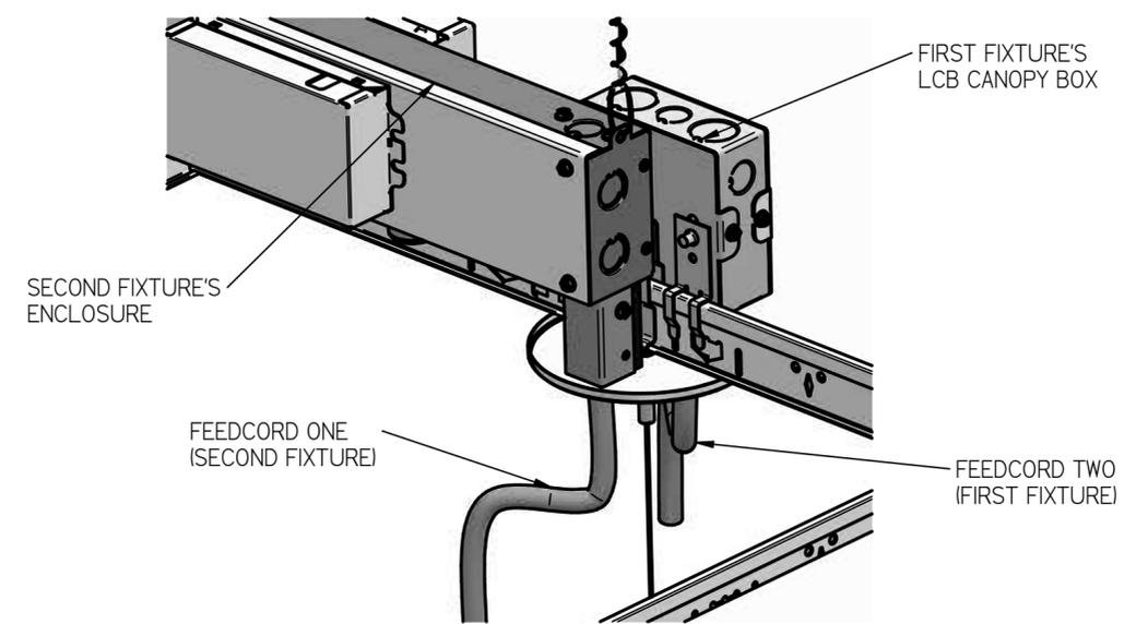
WHEN ROW JOINING FIXTURES THAT HAVE DUAL FEEDCORDS, THE SECOND FIXTURE IN THE ROW CAN SHARE CANOPIES WITH THE FIRST FIXTURE'S LCB CANOPY BOX. ONE FIXTURE CANNOT HAVE TWO FEEDCORDS COMING FROM THE SAME CANOPY.
