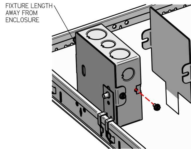
WHEN DUAL FEEDCORDS ARE NEEDED, MOUNT THE PROVIDED LCB CANOPY BOX ON THE TBAR, FIXTURE LENGTH AWAY FROM ENCLOSURE REMOVE COVER AND SET ASIDE.
