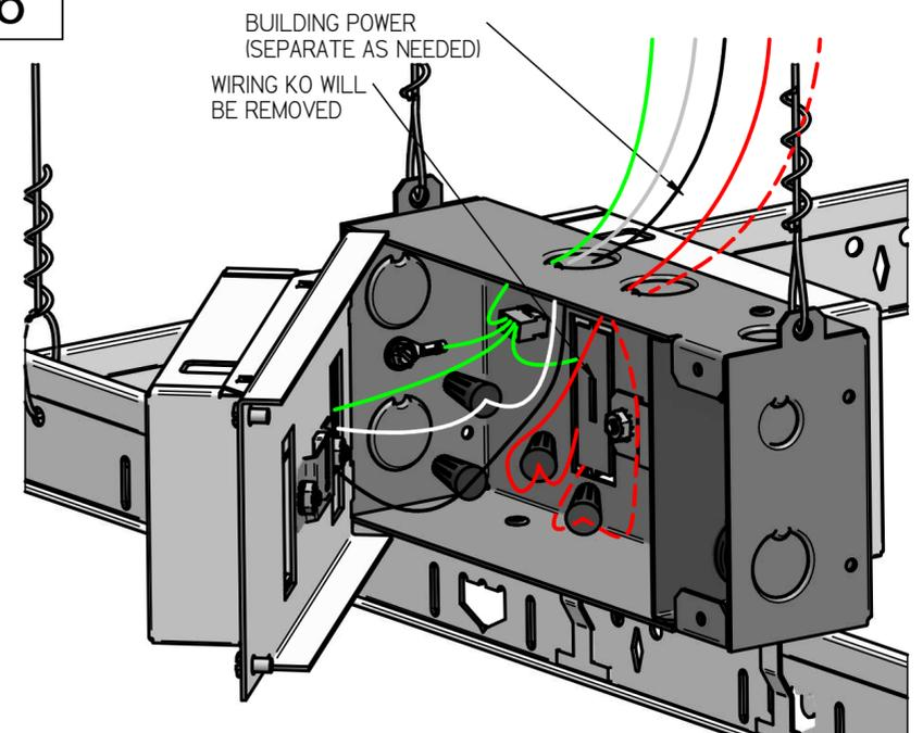
MAKE BUILDING POWER CONNECTIONS IN THE LARGER WIRING COMPARTMENT. ENCLOSURES WITHOUT NX COMPONENTS CAN BE EITHER 1 CIRCUIT OR 2. WIRE ACCORDINGLY BASED ON LABELS AND FIXTURE NEEDS. **NOTE: 2 CIRCUIT SHOWN.**
