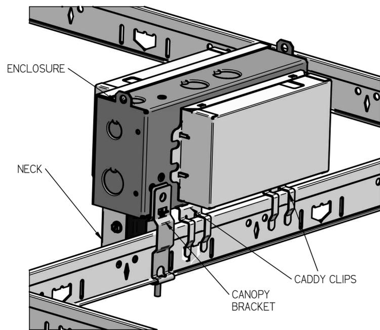
REMOVE CEILING TILE UNDER DESIRED ENCLOSURE LOCATION. MOUNT ENCLOSURE AND CANOPY BRACKET ALONG TBAR. REFER TO DETAIL A ON SHEET 1 FOR TBAR CLIP MOUNTING. **CANOPY BRACKET AND NECK ONLY USED FOR PENDANT FIXTURES.**
