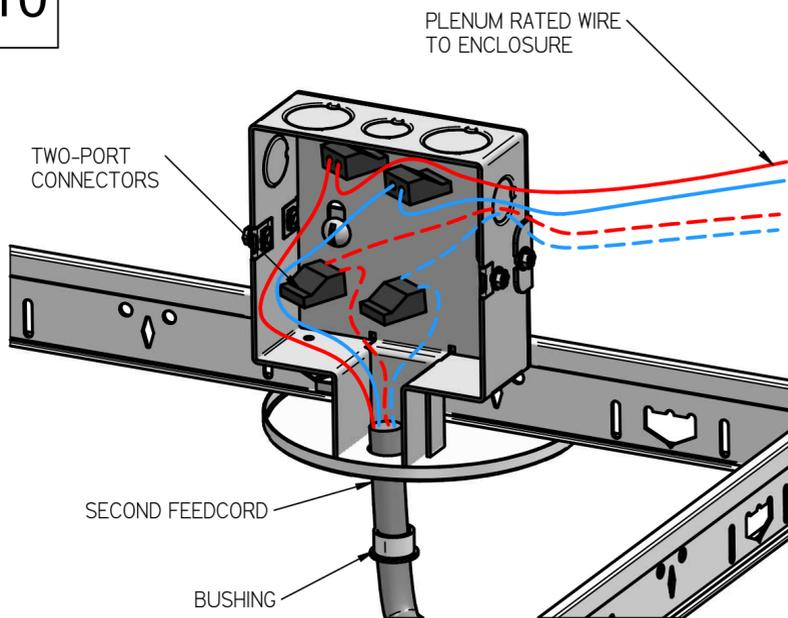
PLACE A BUSHING ONTO SECOND FEEDCORD AND ATTACH TO SECOND CANOPY. ROUTE FEEDCORD INTO CANOPY BOX. USING CONTRACTOR SUPPLIED TWO-PORT CONNECTORS OR WIRENUTS, MAKE CONNECTIONS TO PLENUM RATED WIRING. DEFAULT DIRECT LEDS TO ENCLOSURE FEEDCORD AND INDIRECT TO LCB FEEDCORD.
