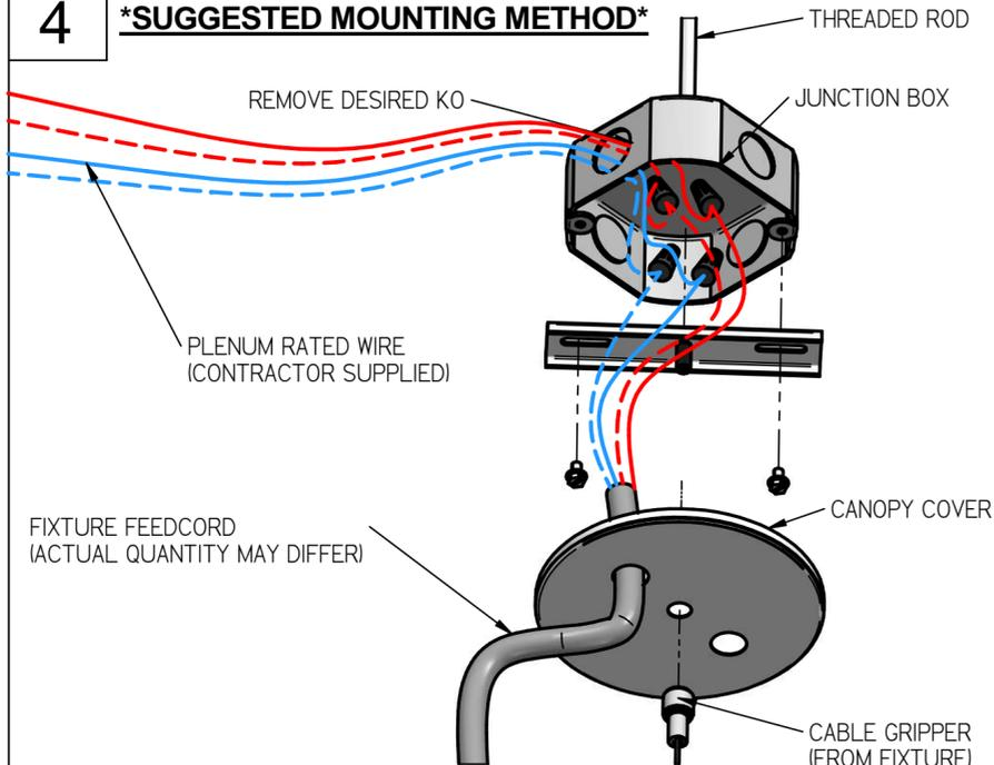
FOR TILE MOUNTED PENDANTS, A CONTRACTOR SUPPLIED JBOX IS REQUIRED TO MOUNT FIXTURE. USE A CONTRACTOR SUPPLIED 18 GA PLENUM RATED WIRE TO MAKE CONNECTIONS INSIDE JBOX. NO NECK IS REQUIRED ON ENCLOSURE. **NOTE: TILE MOUNT METHOD MAY VARY. EVERY FEEDCORD NEEDS A JBOX.**
