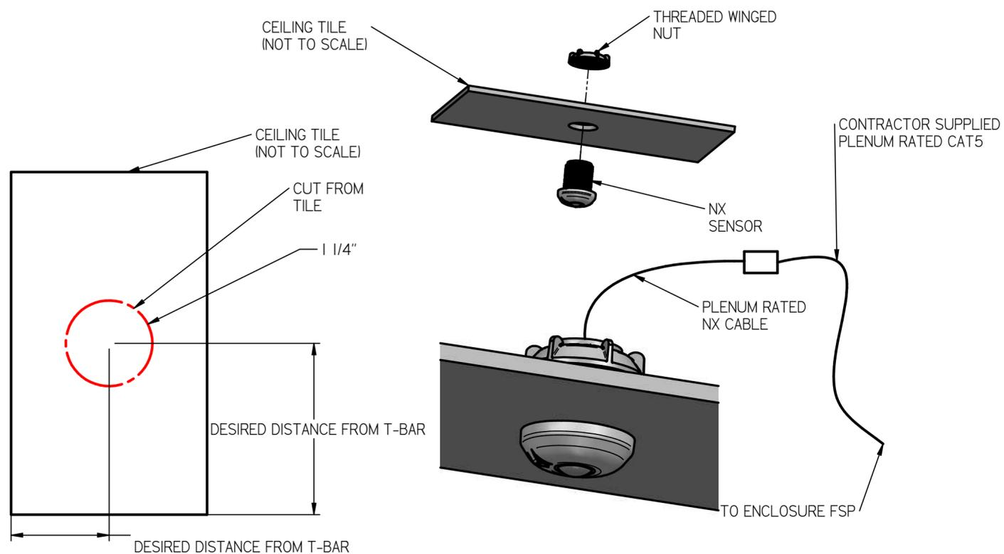
MAKE SENSOR CUT OUT IN CEILING TILE . PLACE SENSOR INTO CUTOUT AND SECURE TO TILE. CONNECT PLENUM RATED NX CABLE TO SENSOR AND CONNECT PLENUM RATED NX CABLE TO ENLCOSURE WITH A CONTRACTOR SUPPLIED CAT5 OF DESIRED LENGTH.
