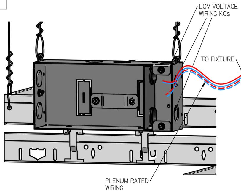
FOR ALL OTHER FIXTURE TYPES, AFTER MOUNTING THE FIXTURE IN PLACE, USE A CONTRACTOR SUPPLIED 18 GA PLENUM RATED WIRE TO CONNECT THE FIXTURE TO ENCLOSURE. NO NECK IS REQUIRED ON ENCLOSURE.
