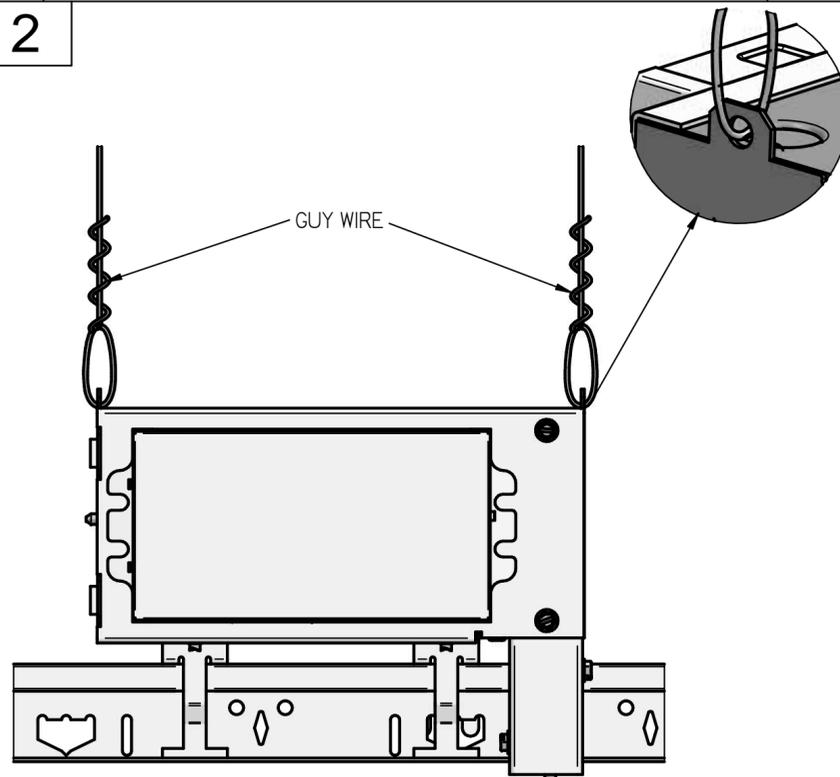
ATTACH THE GUY WIRE (BY SUPPLIER) TO THE TWO SUPPORT LOCATION. REFER TO SHEET 1 FOR MOUNTING DISTANCE WITH THE RESPECTIVE ENCLOSURE SIZE.
