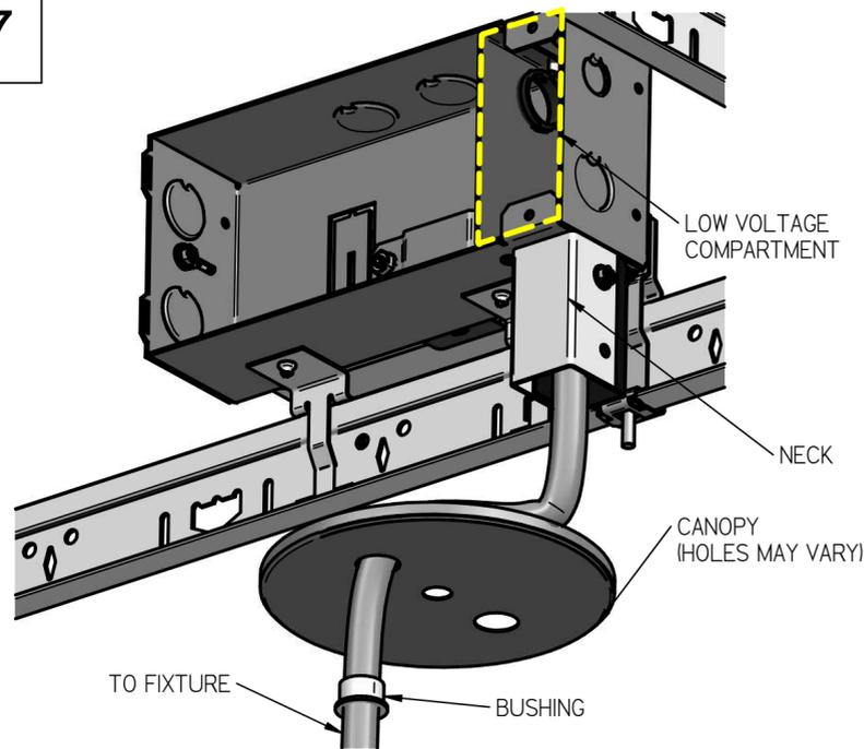
FOR TBAR MOUNTED PENDANT FIXTURES, PLACE BUSHING AND CANOPY COVER ONTO FEEDCORD. ROUTE FEEDCORD INTO ENCLOSURE THROUGH NECK. ATTACH BUSHING TO CANOPY. IF USING SMALL ENCLOSURE, OR ONLY INSTALLING ONE FEEDCORD, WIRE FEEDCORD TO ENCLOSURE AND REPLACE COVER AND SKIP TO STEP 12.
