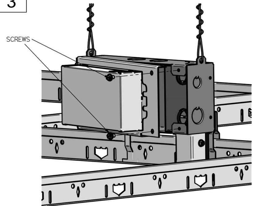
REMOVE SCREWS AND COVER WITH THE 1/4" SOCKET. **DO NOT TUG ON COVER OR PULL TOO FAR AWAY FROM ENCLOSURE.**
