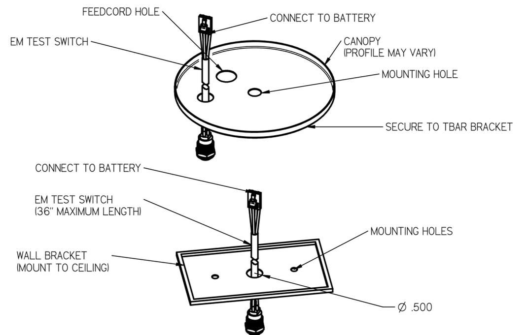
TOP IMAGE: THIS METHOD IS ONLY FOR PENDANT FIXTURE MOUNTED ON THE TBAR. SECURE EF SWITCH TO CANOPY PLATE AS WITCH HEX NUT. CONNECT SWITCH TO BATTERY.
