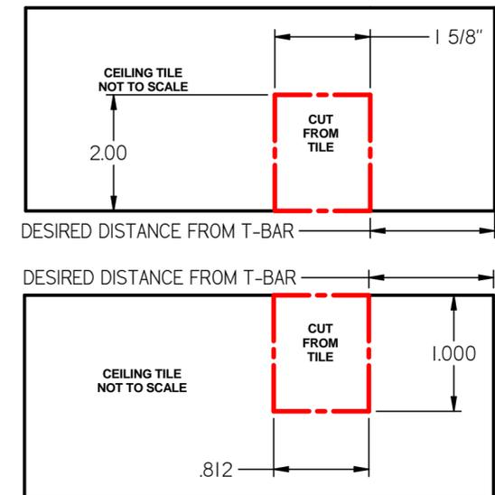
MAKE CUTS ON CEILING TILES AS NEEDED. REFER TO ENLCOSURE LAYOUT ON SHEET 4 TO CUT PROPER TILES. DESIRED DISTANCE FROM TBAR DIMENSION NEEDS TO BE EQUAL ON BOTH TILES. PLACE CEILING TILE BACK IN CEILING AND MOUNT FIXTURE USING THE 70L PENDANT INSTALLATION GUIDE. FOR TILE MOUNT, CUT A HOLE IN THE TILE BASED ON JUNCTION BOX/OTHER MOUNTING METHOD'S DIMENSIONS.
