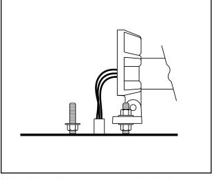
Mount hinged base to any two anchor bolts depending on hinge direction desired. Secure with nuts and washers.
