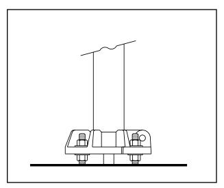
Feed input leads through pole bottom and out hand-hole. Tilt pole up and onto the two unused anchor bolts. Secure with nuts and washers. Check conduit height for possible interference.
