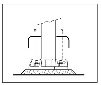
Level pole if necessary. Secure pole with nuts and washers. Pole base must have full contact with foundation by grouting. Make wire connections at handhole and install handhole cover. Attach base cover to pole base.
