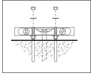
Anchor bolts must be installed as per installation guide supplied with anchor bolts. All bottom nuts and washers must be leveled as shown.
