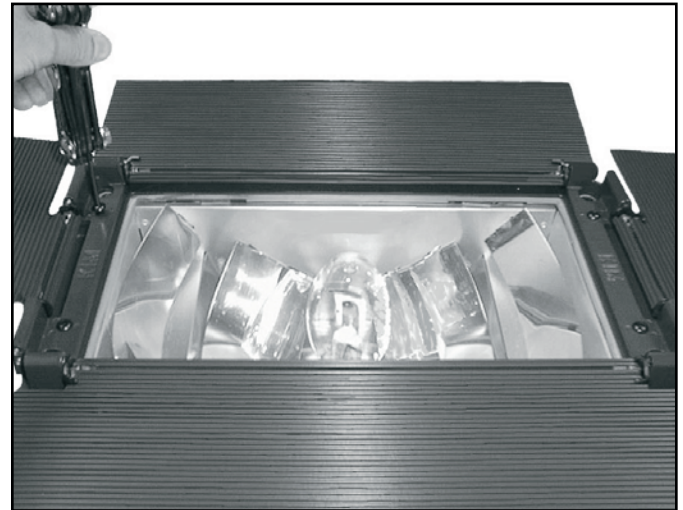
2. Install Barn Door Assembly with (4) 10-32 x 1/2" Button Head screws.
