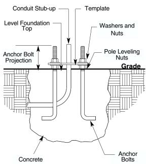
Concrete foundation to be designed according to local soil conditions.
