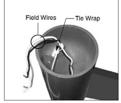
**4.** Pull field wires through pole tenon into slipfitter and through tie wrap. Tie field wires into a knot or back loop through tie wrap.
