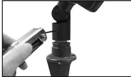
8. Loosen set screw, adjust fixture rotation, and tighten set screw.
