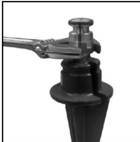
2. Tighten coupling onto mounting device.
