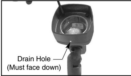
7. Replace lens (convex side out) fitting lens gasket assembly into the recess on fixture body. Replace light shield over lens after making sure the drain hole is down, so water will not stand on lens. Tighten opposing screws progressively and evenly.
