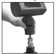
2. Attach fixture unto coupling. Connect fixture cable to main system cable with a KLV410 Sealed Connector (Part No. 95484).
