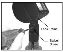
To adjust backtilt up to maximum, loosen swivel screw being careful not to disengage threads. Hold fixture at desired angle and firmly tighten swivel screw.
