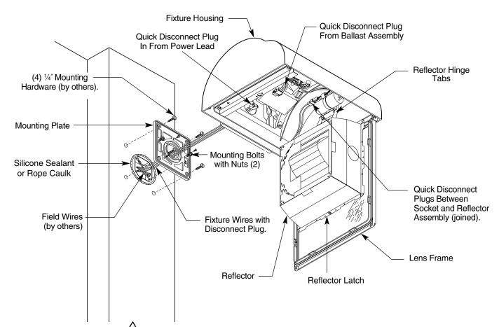
**Installation Instructions:**  $\angle$ !\text{\text{ Make certain electrical supply is **OFF** before starting installation.
