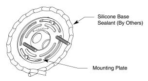
Apply silicone base sealant (by others) about 1" away from mounting plate to prevent water intrusion. **NOTE:** In conformance with UL Standard 1570, 1571, & 1572, a silicone base sealant must be used between fixture and supporting wall.
