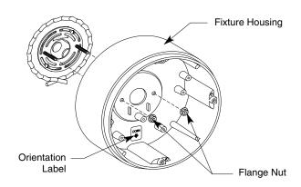
Install fixture housing to mounting plate. (Note orientation label on inside of housing.) Pull electrical wires into housing. Press housing to wall, rocking gently to seal caulking. Use flange nuts to tighten housing to wall. Do not over tighten.
