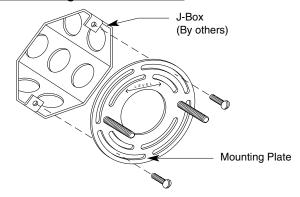
Install mounting plate to J-box using screws provided with J-box. Make sure that threaded studs projecting from plate are **horizontally level**.
