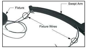
4. Install fixture to swept arm. Pull wire through swept arm and out arm access opening. Push wire into pole and out the top of the slipfitter.
