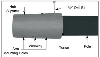
2. Remove and drill recess for each of the bottom set screws. Use a <sup>3</sup>/<sub>6</sub>" drill bit. Replace set screws and tighten until hub is secure.
