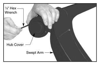
6. Install hub cover and secure with screws.
