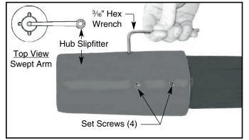
Slide hub slipfitter over tenon. <u>Important!</u> Orient slipfitter mounting holes in direction of Swept Arm assembly and tighten (4) set screws using a <sup>3</sup>/<sub>16</sub>" hex wrench. (See "top view" above.)
