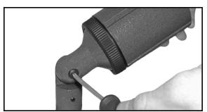
**5.** Adjust angle using swivel screw. Retighten after adjustments.
