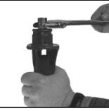
Tighten coupling onto mounting device. (See KIM Installation Instructions for Low Voltage Mounting Options, part no. 95488.)
