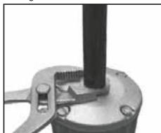
3. Position fixture & tighten locknut with adjustable wrench.
