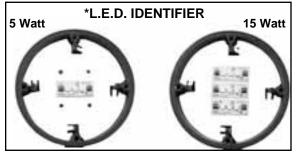
8. \*L.E.D. identifier - both are available in 120 volt or 277 volt input. Reference label on side of driver component or lamp label to determine.
