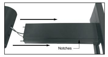
4. Slide arm onto studs with notches down.
