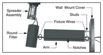
3. Feed supplied wiring through wiring hole in round fitter, arm, and wall mount cover.
