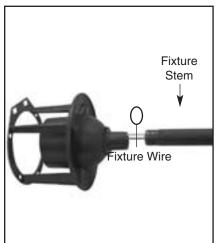
Feed wires through stem (short threaded end first), thread stem into fixture body and tighten securely.
