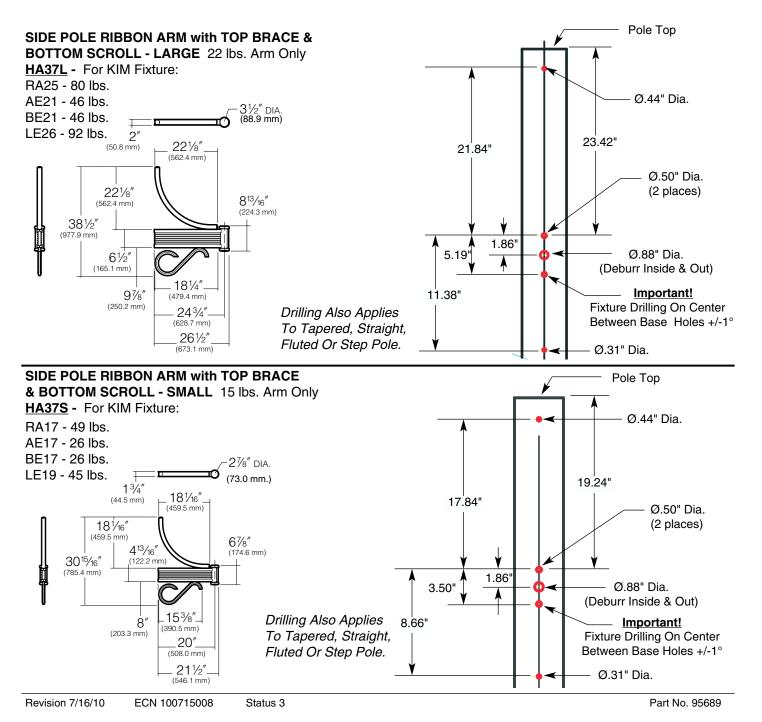
**Fixture mounting arrangements:** The desired mounting arrangement will determine the required position of drilling on pole by others. Mounting arrangement is determined by KIM catalog number.
