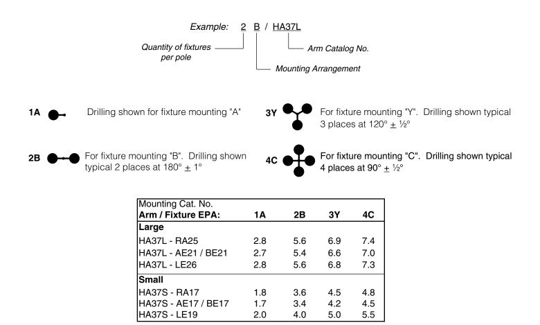
**Note:** For proper drilling be sure to note fixture orientation to anchor bolts. Select one of the orientations suited to your pole and keep consistent for all poles the same. Drawings below show proper orientation for fixture mounting arrangement "A". Arrangements "B", "C", and "Y" are typical.
